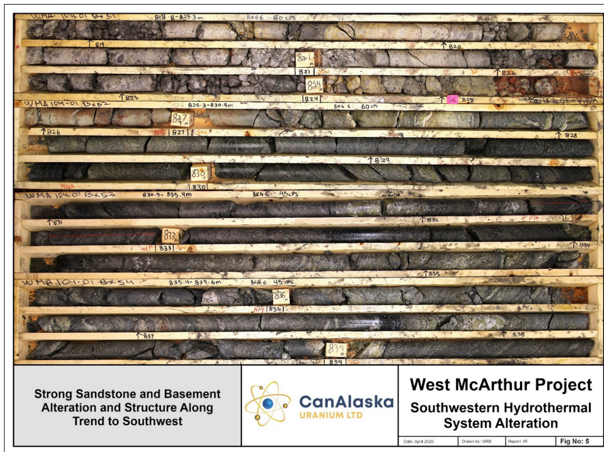
Figure 5 – Strong Sandstone and Basement Alteration and Structure to the Southwest Along the C10S Corridor. Sandstone Fault Zone with Broken and Blocky Core with Associated Strong Quartz Dissolution, Bleaching, and Intense Sooty Pyrite Alteration Resulting in Locally Poor Core Recovery. Basement Consists of Graphitic Pelite with Re-Activated Structure and Associated Chlorite, Clay, Bleaching, and Quartz-Carbonate Alteration. Drillhole WMA104-01.
